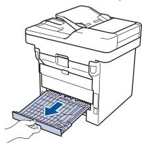
4. Pull the jammed paper out of the machine or out of the 2-sided tray.
